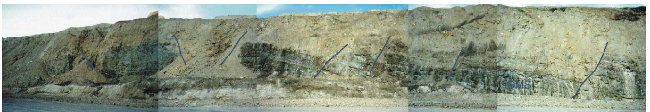
Figure 19 Moderately dipping normal faults forming in response to accommodation above a major thrust fault (Goonyella).
