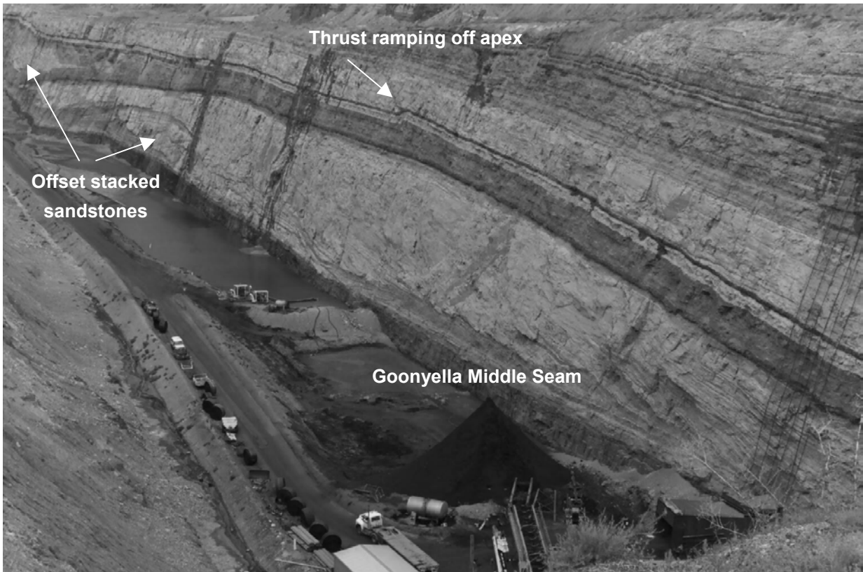
Figure 48 Lenticular cross-section of 35m thick amalgamated crevasse-splay channel unit dominated by medium- to coarse-grained cross-stratified lithic sandstone. Goonyella Mine Ramp 4 South high wall (75m high).
