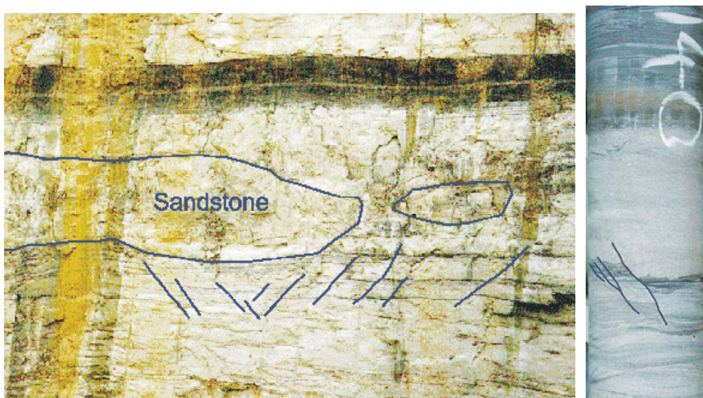
Figure 16 Small normal faults below a geotechnically massive sandstone body, in outcrop and in drill core (Goonyella).
