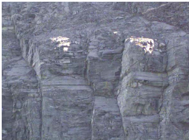
Figure 24 Major vertical joint set in sandstone unit (Saraji).
