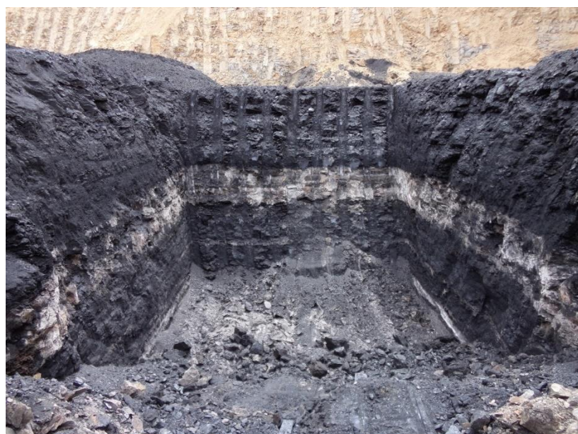
Figure 59 Photograph of the Yarrabee Tuff within the Pisces Seam, exposed at Foxleigh Mine test pit. (Sample and image courtesy of Aastha Sharma, AngloAmerican)
