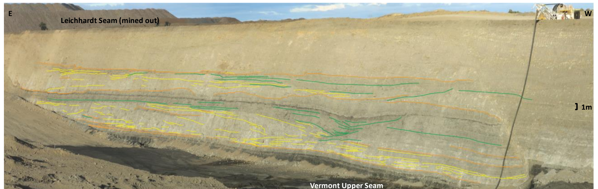
Figure 38 Mining exposure of the YT to Leichhardt interburden at Daunia showing sedimentary features highlighted in yellow (sandstone) and green (siltstone).
